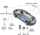
Intelligent Connected Vehicle Antenna
